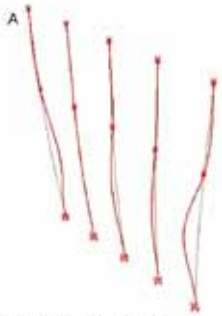
Model 1 - "A" Elements Column Demand: 56,000KN Buckling Load (Capacity): 25,000KN
