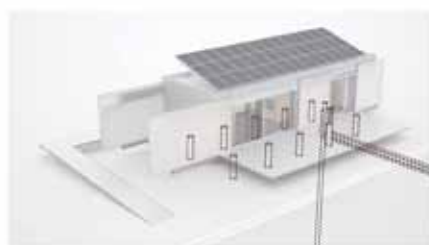
A. SITE PREPARATION: Utilities are installed, foundations are set, and geothermal is loop drilled.
