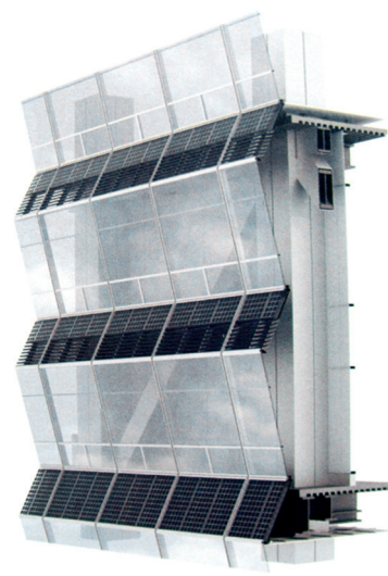
图55 墙面光伏组件倾斜30°
