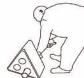
Pvc pipes are manually removed after casting
