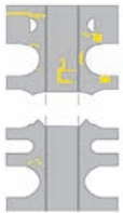
The location of cracks was mapped and injected with concrete to stabilize the bridge
